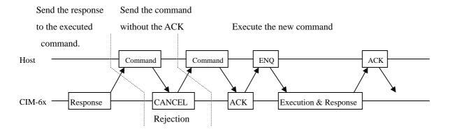
The terminal should ignore the command received before it sends the ACK packet, send the CANCEL packet. The second command will be treated as the ACK packet and executed with no ACK.
